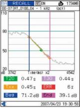
Measurement results of reverberation time decay curve
