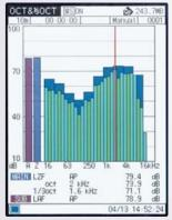
Analysis mode screen (Simultaneous 1/1 & 1/3 octave band display)
